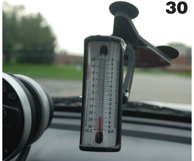
Deceleration after installation of the new brakes was 23 feet per second per second. This test was performed after only six 35-mph stops with the new brakes. After the brakes are seated in, there should be an additional 15% to 20% improvement. UD
