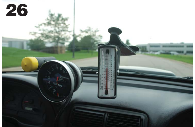
This windshield-mounted gauge measures deceleration in feet per second per second on the left scale and meters per second per second on the right. Although it's not as high-tech as a GPS computerized deceleration read-out or a dyno test, it does clearly show a vehicle's stopping ability in terms of deceleration rate.
