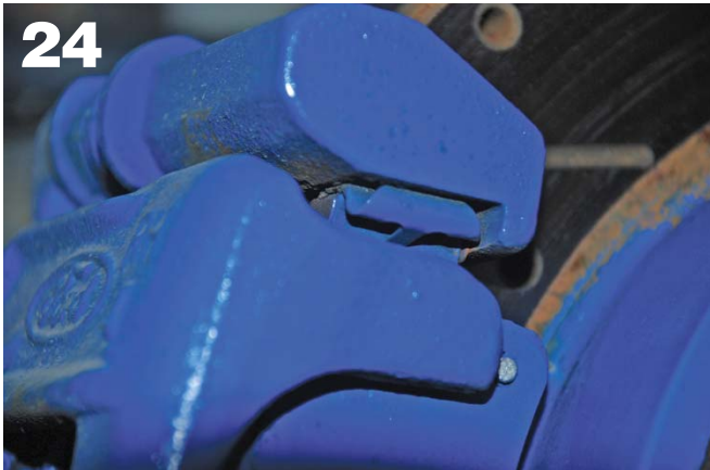
Look carefully at the anti-rattle-clip pad tensioner, indicative of the underlying rust problem.
