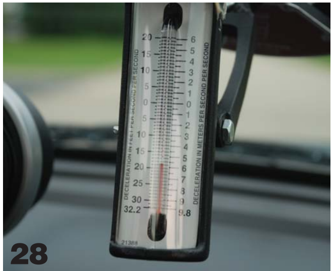
The gauge shows that the vehicle's best deceleration rate before the brakes were replaced was 19 feet per second per second.
