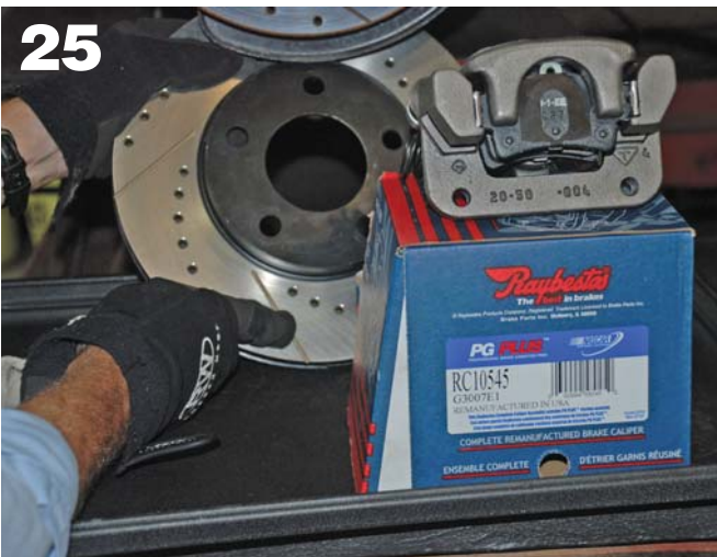
New drilled and slotted rotors, premium pads and quality calipers with new brackets and hardware are the cure for this vehicle's braking problem.
