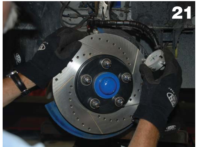
Using a dial indicator, measure runout on the new rotor. On a drilled and slotted rotor you can't have the contact point of the runout gauge dipping into the slots or holes, so take your runout reading at the outer edge.
