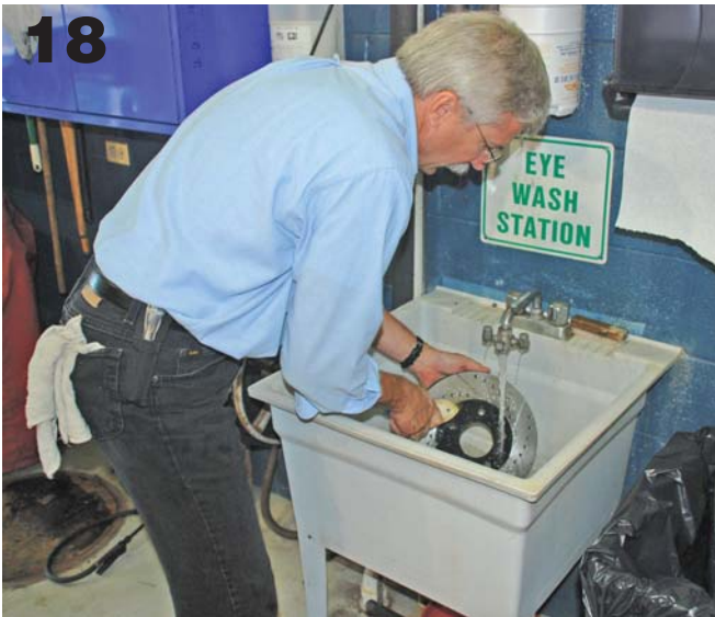
As any good machinist will tell you, washing with soap and water should be the final step in cleaning a rotor. The soap lifts off any remaining particles so you can flush them off the surface.
